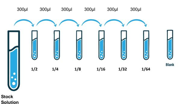
Note: The standard solutions are best used within 2 hours. The standard solution series should be kept at 4°C for up to 12 hours. Or store at -20 °C for up to 48 hours. Avoid repeated freeze-thaw cycles.
